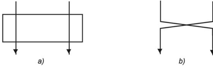
FIGURE 3.8 Schematic representation of the P_{2/1} block in the form of two elementary bijective transformations carried out over a 2-bit vector (x_1, x_2) provided that v = 0 (a) and v = 1 (b).
